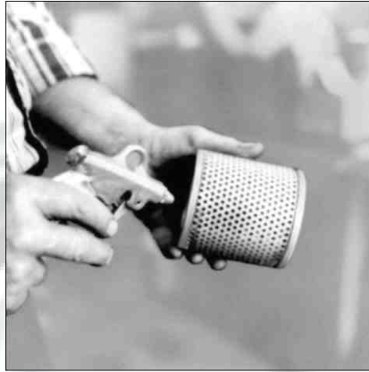
Cleaning the air filter
